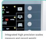
Integrated high precision scales measure and record weight increments of the child in a table and graph.
